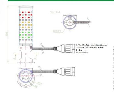
IP67 with water jets falling directly on the top of the column
